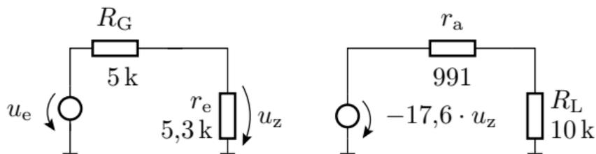
$$\begin{aligned} \frac{u_{RL}}{u_e} &= \frac{r_e}{R_G + r_e} \cdot (-17,6) \cdot \frac{R_L}{r_a + R_L} \\ &= 0,534 \cdot (-17,6) \cdot 0,910 = -8,55 \end{aligned}$$
