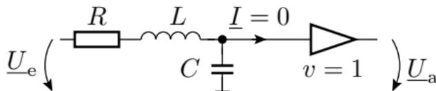
$$\frac{1}{1 + j\omega RC - \omega^2 LC} = \frac{1}{1 + a_i \cdot \frac{j\omega}{2\pi f_0} + b_i \cdot \left(\frac{j\omega}{2\pi f_0}\right)^2}$$
