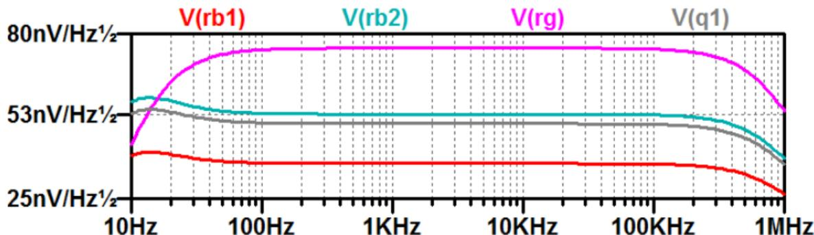
$$2 \quad SNR = \left( \frac{1 \text{ mV}}{\sqrt{2} \cdot 13 \mu\text{V}} \right)^2 \approx 2960$$
