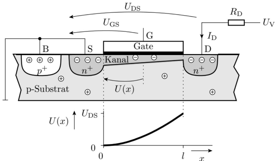
$$I_D = C_1 \cdot \mu \cdot (U_{GS} - v_{to} - U(x)) \cdot \frac{dU(x)}{dx}$$
