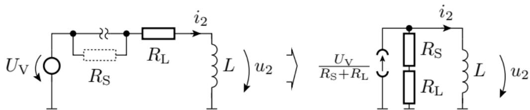
$$I_2^{(+)} = \lim_{R_S \rightarrow \infty} \left( \frac{U_V}{R_L + R_S} \right) = 0$$
