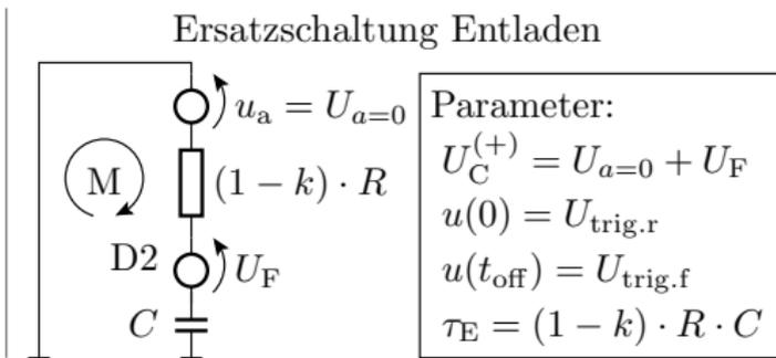
$$t_{\text{off}} = (1 - k) \cdot R \cdot C \cdot \ln \left( \frac{U_{a=0} + U_F - U_{\text{trig.r}}}{U_{a=0} + U_F - U_{\text{trig.f}}} \right)$$
