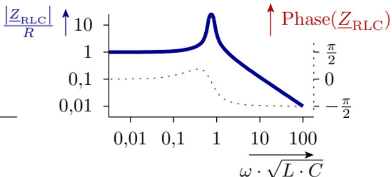
$$\begin{aligned} \underline{Z}_{\text{RLC}} &= \underline{Z}_{\text{RL}} \parallel \underline{Z}_{\text{C}} = \frac{1}{\frac{1}{R+j\cdot\omega\cdot L} + j\cdot\omega\cdot C} \\ &= \frac{R + j\cdot\omega\cdot L}{1 + j\cdot\omega\cdot R\cdot C - \omega^2\cdot L\cdot C} \end{aligned}$$
