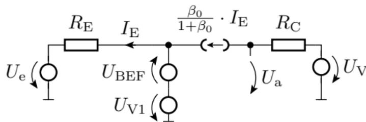
$$\left| \begin{array}{l} R_E = 220 \, \Omega \\ R_C = 1 \, \text{k}\Omega \\ U_V = 5 \, \text{V} \\ U_{CEX} \approx 0,2 \, \text{V} \\ U_{BEF} \approx 0,7 \, \text{V} \\ \beta_0 = 100 \end{array} \right.$$
