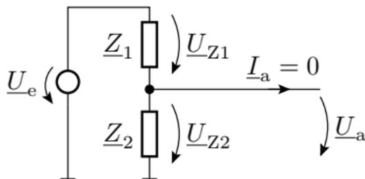
$$\underline{U}_a = \underline{U}_e \cdot \frac{\underline{Z}_2}{\underline{Z}_1 + \underline{Z}_2}$$
