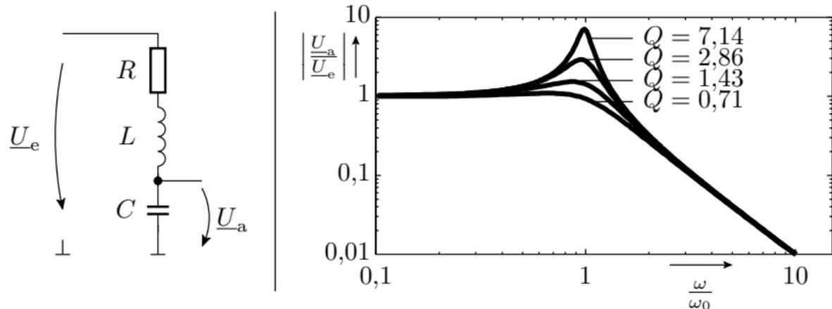
$$\underline{U}_a = \underline{U}_e \cdot \frac{\frac{1}{j \cdot \omega \cdot C}}{R + j \cdot \omega \cdot L + \frac{1}{j \cdot \omega \cdot C}} = \underline{U}_e \cdot \frac{1}{1 + j \cdot \frac{\omega}{Q \cdot \omega_0} - \left(\frac{\omega}{\omega_0}\right)^2} \quad (1)$$
