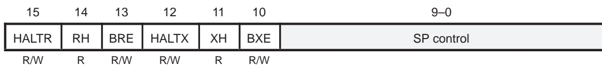
Figure 9–36. BSP Control Extension Register (SPCE) Diagram — ABU Control Bits
